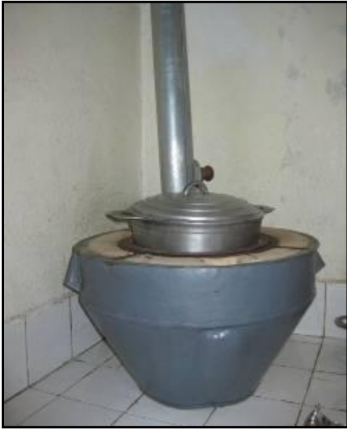
Figures 5.24 to 5.25: The modified wood stove, or fatana pipa stove
