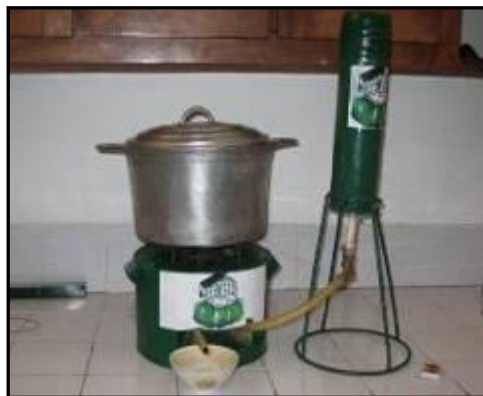
Figure 5.11: Front view of the ISPM Stove
