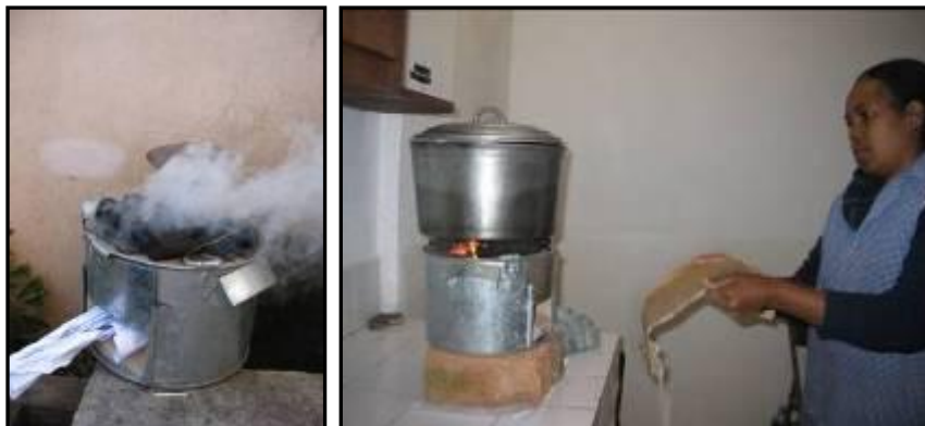
Figure 5.15 (left): The MCS is lit with wood or paper and takes 10 to 12 minutes to kindle.
