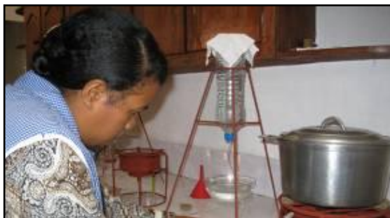
Figure 5.6: Regulating the fuel flow to the stove
