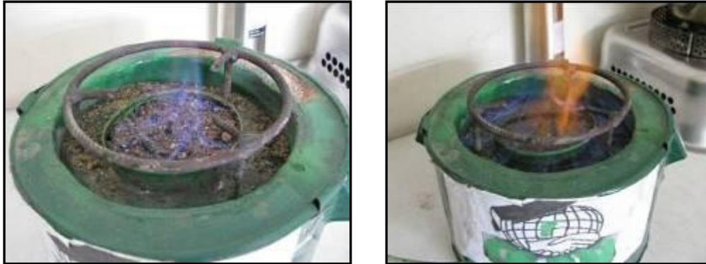
Figure 5.14 (left): Burner showing coarse sand and small stones and ample well around burner. (right): Ethanol in the burner and the well on fire. The cooks used the stove with burner and well (trough) lit. This resulted in a higher rate of fuel consumption
