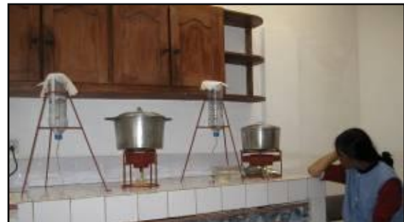
Figure 5.7: The single and multiple burner stoves during the water boiling tests
