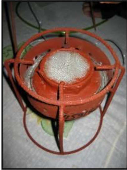
Figure 5.4: Top view of a single stove burner
