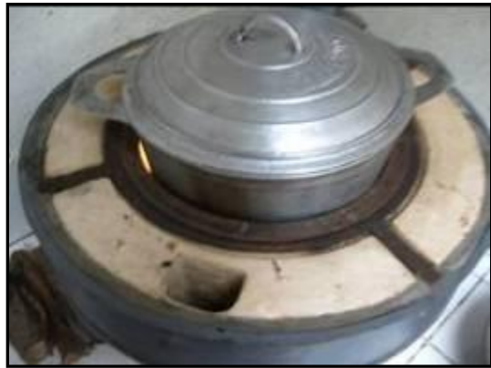
Figures 5.24 to 5.25: The modified wood stove, or fatana pipa stove
