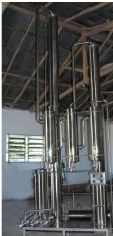
Distillation unit: 1000 litres per day
