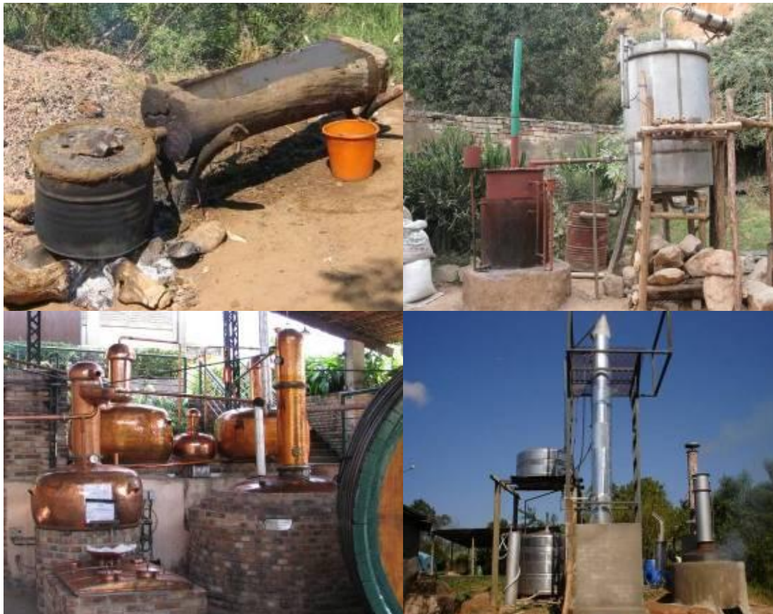
Figure 2.3: Artisanal and Batch Stills
